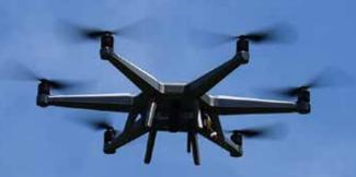
Specifications Range: 2.5km plus Speed: 15m per second Endurance: 20 minutes Weight: ~5kg
