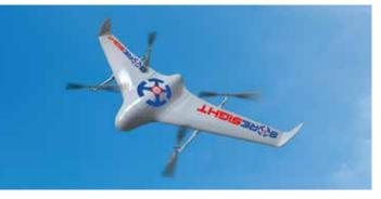
Specifications Range: 5km plus Speed: 30m per second Endurance: 25 minutes Weight: 7kg Size: 2200mm (W) x 800mm (L)
