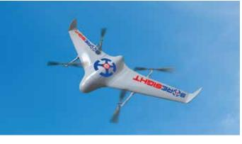
Specifications Range: **5km plus** Speed: **30m per second** Endurance: **25 minutes** Weight: **7kg** Size: **2200mm (W)** x **800mm (L)**
