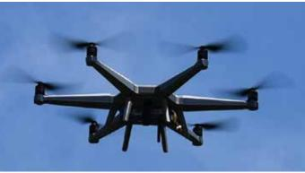
Specifications Range: **2.5km plus** Speed: **15m per second** Endurance: **20 minutes** Weight: **~5kg**
