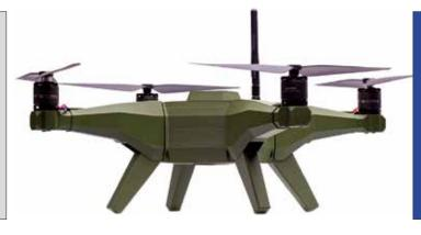
Specifications Range: **2.5km plus** Speed: **18m per second** Endurance: **20+ minutes** Weight: **1.3kg**
